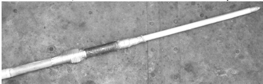
Next, with the foreshaft in place, I drill a small hole completely through both the bamboo and the aluminum shaft inside. I place this hole carefully, directly behind the wrapping on the front of the dart. I then insert a small length of copper wire and bend it back on either side of the shaft, with the ends facing the fletching
